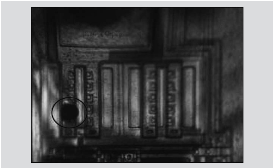
Figure 13.13 Liquid Crystal Thermography uses temperature sensitive chemicals and polarized cameras to detect hot spots on the die surface.
