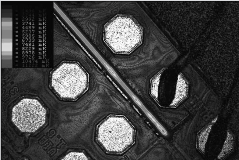
Figure 13.12 Fluorescent Microthermal Imaging produces static thermal maps of surfaces or/and localizes “hot spots”.
